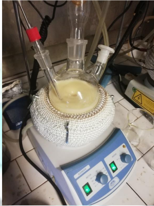
Figure 12. Three-neck round bottom reactor with transesterification reaction taking place.
